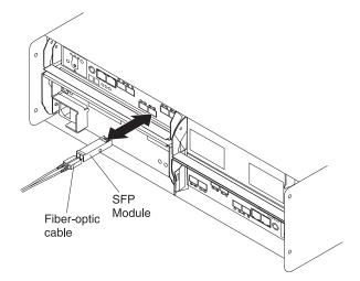
Figure 85. Replacing an SFP module
